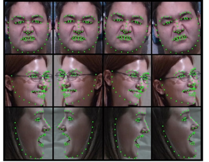
Fig. 3. Image rotation and mirror transformation in SIFT extraction process. The first column contains original images. The images in the second column are under mirror transformation. The images in the third and fourth columns are rotated ten degrees clockwise and counterclockwise respectively.
